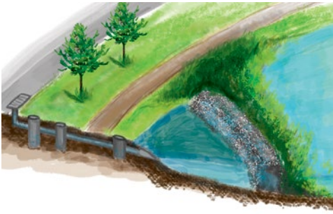
Figure 15. Buffer zone with biogeochemical barrier for the pre-treatment of water conveyed directly to the reservoir: schematic representation and pilot project in the ponds of Arturowek in Lodz
